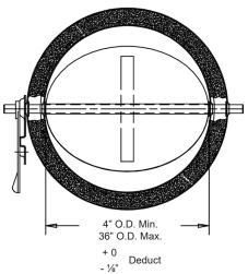
Damper fits inside both skins of dual wall spiral duct. Note that O.D. and I.D. are 1/8" undersized.
